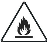
Caution: Risk of fire
